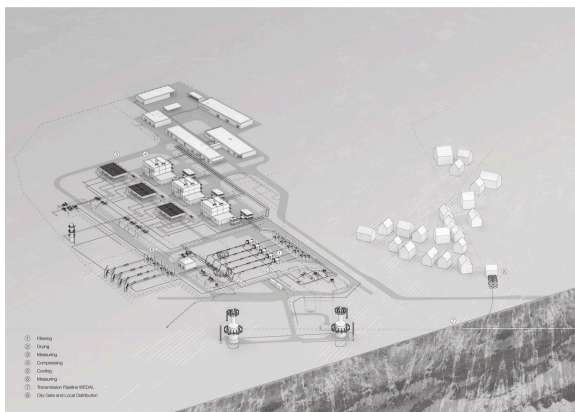
COMPRESSOR STATION ALONGSIDE THE WEDAL PIPELINE IN WÜRSELEN (GERMANY) Source: Zeelink, 2017 [ https://www.zeelink.de/ ]
