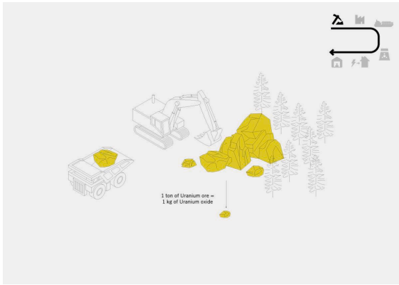
URANIUM EXTRACTMENT FROM THE MINE
