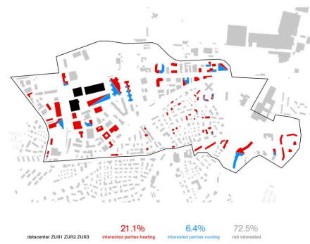
The Airport City perimeter and its possible interested parties in waste heat and cold.
