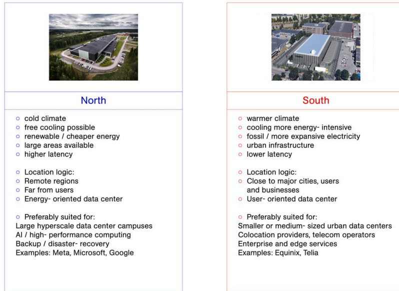
Comparison of typical data centre location strategies: Source: Meta Platforms Inc., 2023; Equinix Inc., 2023.
