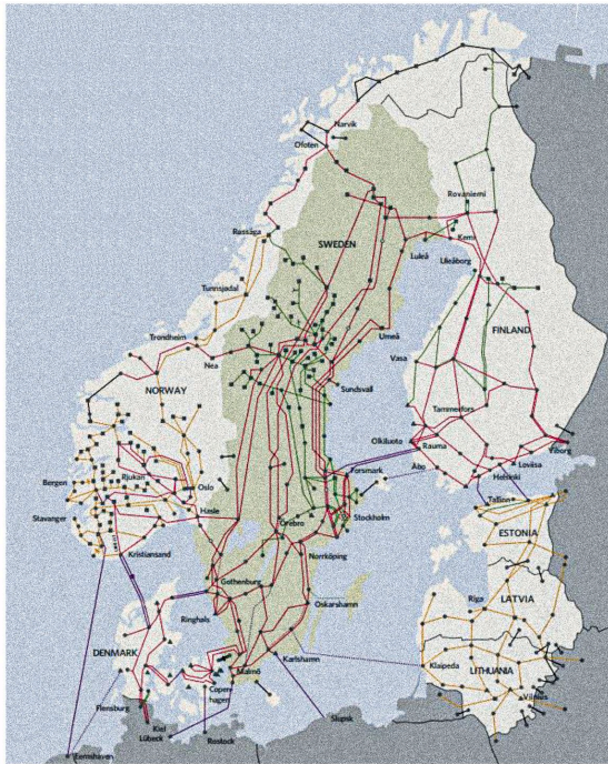
Nordic high-voltage electricity transmission network
