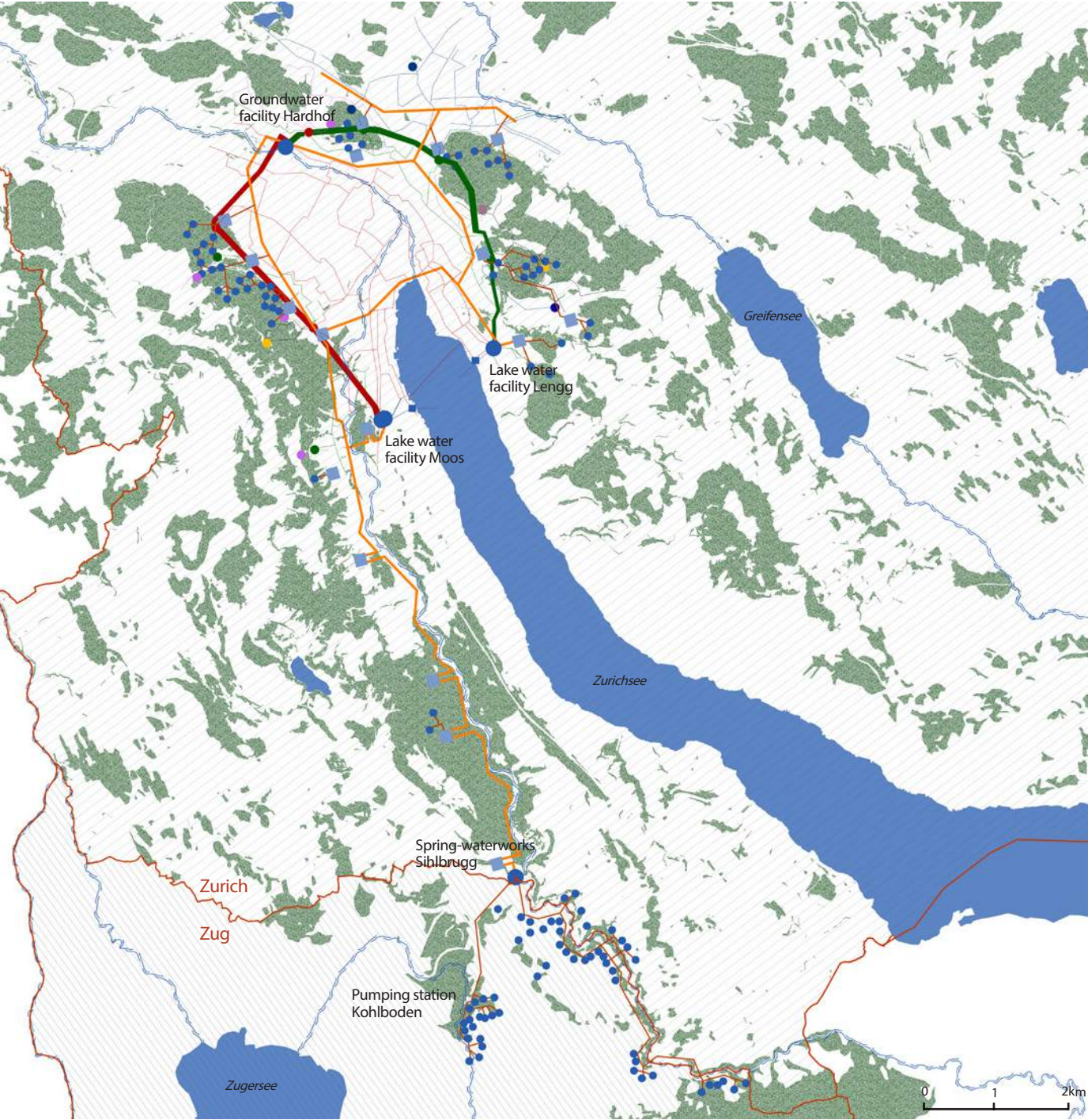
fig. 29 Zurich headwaters Water from 120 spring sources in the Sihl- and Lorze Valley flows into the water supply network of the city of Zurich. 90% of
