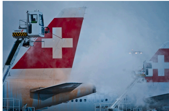
De-icing airplanes at the airport Zurich. Source: Zurich Airport.
