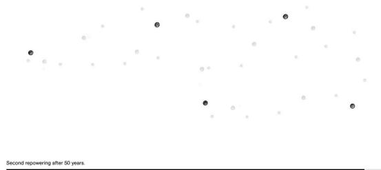
**WIND TURBINES.** The number of turbine decreases while the power capacity is increased.
