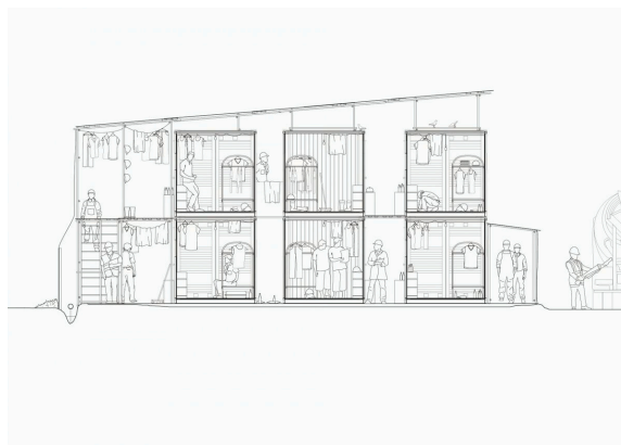
A TEMPORARY DORMITORY WITH CARGO CONTAINERS. ASIA SQUARE CONSTRUCTION SITE, SINGAPORE.
