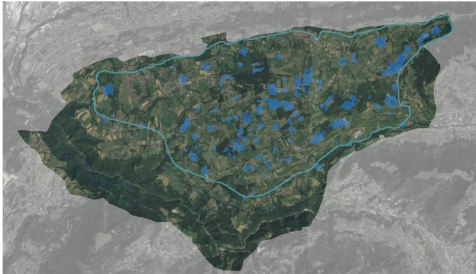
The impluvium takes 35 km<sup>2</sup> of the plateau's area and is defined by topography and wetlands, that are spread and take in about 10 % of the surface but through topographical disposition they'll absorb 30 % of the fallen water. With the turn of the Millennium the focus of Evian water shifted more and more to the backside of Evian-les-Bains and a lot of protectional labels and facilities were launched. At the same time the company extended its product range.
