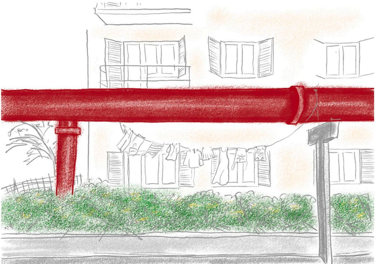
When heat sources are uncertain, flexibility is essential. Above-ground pipelines provide a cheaper, quicker and more adaptable means of connecting fluctuating energy producers, such as data centres, to the urban infrastructure, making energy flows visible and responsive.
