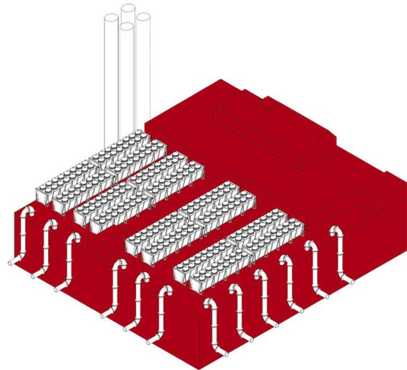
AXONOMETRY OF A DATA CENTRE MADE VISIBLE THROUGH OVERHEAD DISTRICT HEATING PIPES
