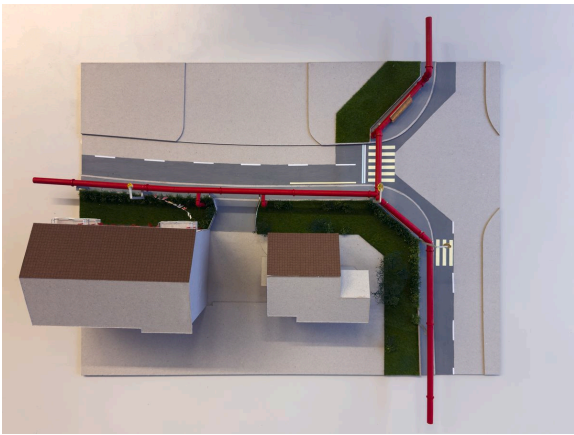
THE THERMAL NETWORK'S END USERS, TOP VIEW Photograph and model: the authors, 2025.
