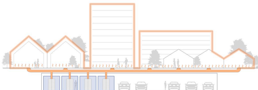
CONCEPTUAL SECTION OF MODULES HEATING THE COMMUNITY The micro data centre modules located in an underground car park heat the buildings above via an internal grid. Drawing: the authors, 2025.
