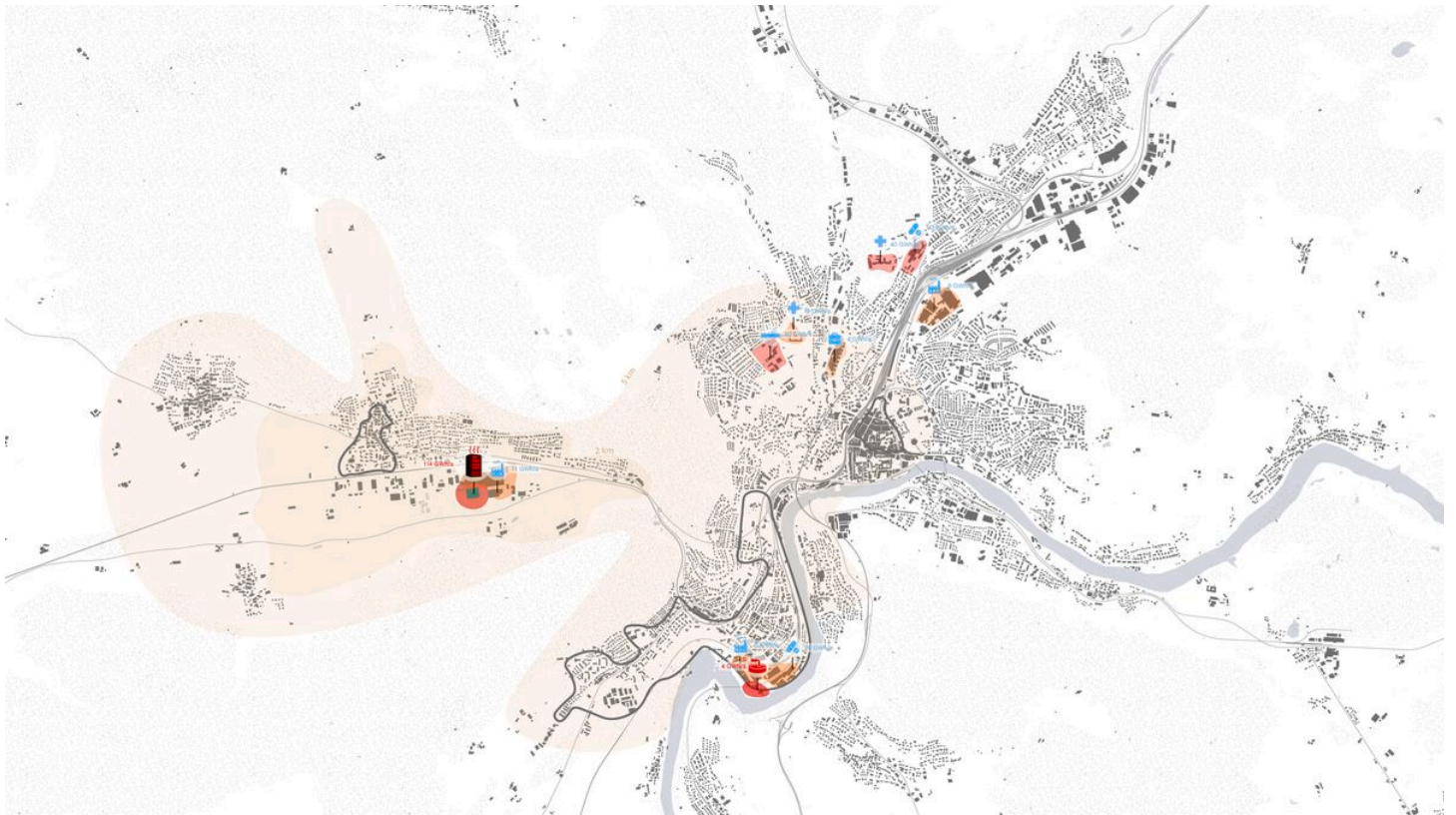
Local thermal relationships in Beringen: the proposal investigates how different producers and consumers can become spatially connected through local and regional heat exchange systems. Drawing: the authors, 2026.
