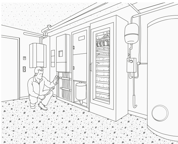
Server integrated in a utility room.
